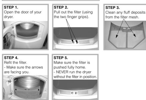
Failure to clean the filter after EVERY drying cycle will affect the drying performance of your machine.
